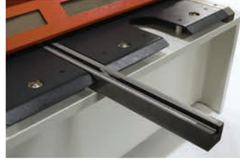
Cetveli, stoperli ve T-kanallı ön destek kolları T-slotted front support arms with scale and flip-stop
